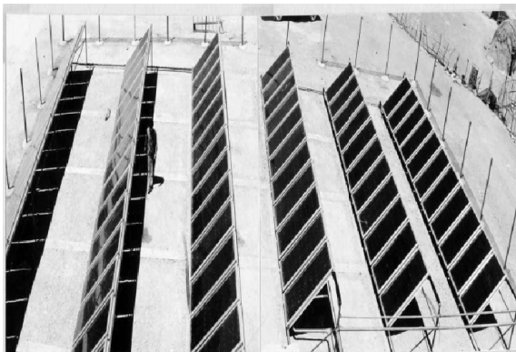
Fig. (9): Full assembly solar collector
