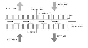
Fig. (2): Layout of a heat pipe.
