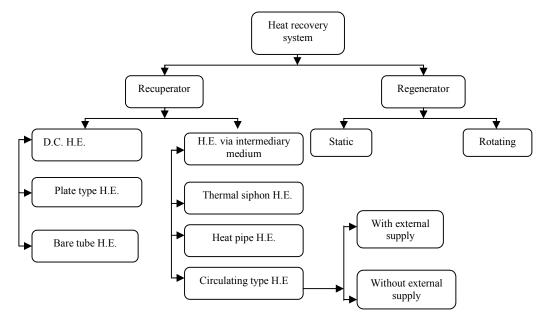
Fig. (1): Classification of heat recovery system
