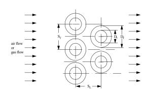
Fig.(8): Arrangement of heat pipes in heat exchanger
