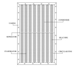
Fig. (3): Heat pipe heat exchanger
