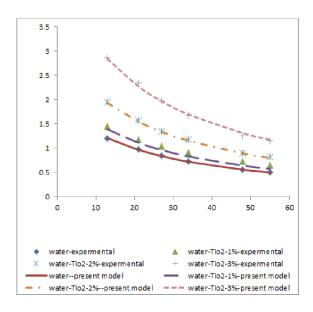
Fig. (2): Variation of relative viscosity  $(\mu_{eff}/\mu_f)$  with temperature for TiO<sub>2</sub>-water system for various volume fractions and its comparison with model prediction.
