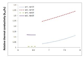
Fig. (6): Variation of relative thermal conductivity (k<sub>eff</sub>/k<sub>f</sub>) with (t/d<sub>p</sub>)
