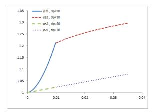
Fig. (4): Variation of relative thermal conductivity  $(k_{eff}/k_f)$  with volume fraction ( $\phi$ )
