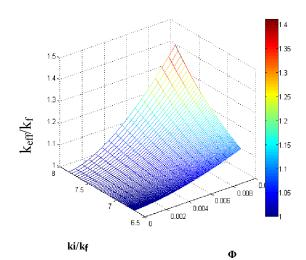
Fig.(8): Variation of relative therm.....ductivity ( $k_{eff}/k_f$ ) with ( $\phi$ ) and (ki/kf) for ( $\phi$ <1%, dp<20nm) region.
